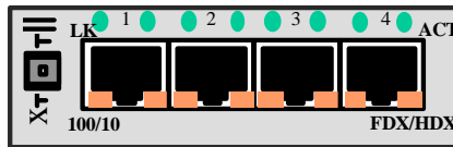
Figure 4.3 : Up-link push-button on RJ-45 quad-port
