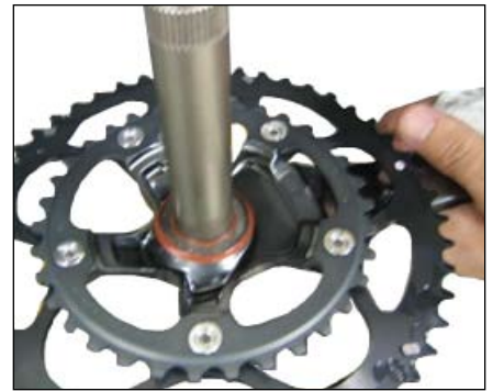
Figure 33. Sliding the bearing cover onto the axle
