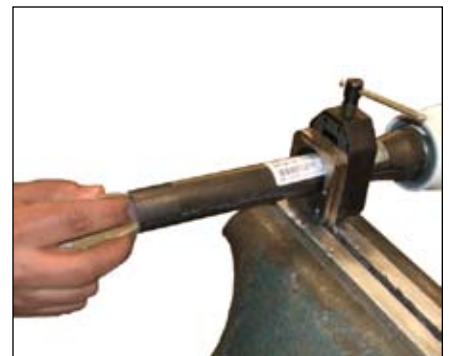
Figure 4. Smooth the inside of the steerer with fine-grit sandpaper
