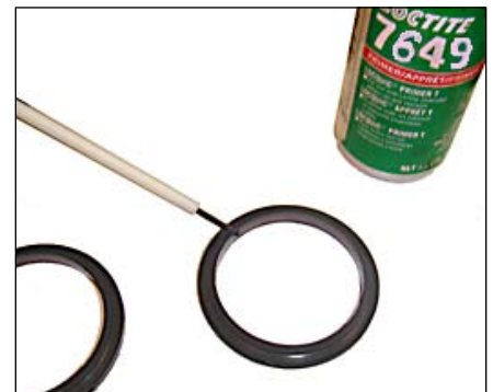
Figure 40. Applying Loctite primer to the outer step of the bearing cups
