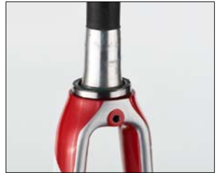
Figure 6. Lower bearing on fork crown
