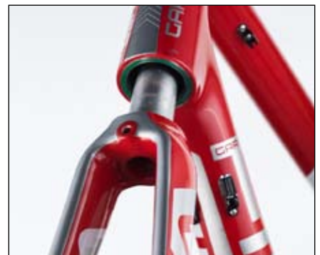
Figure 8. Inserting the fork through the head tube
