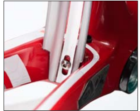
Figure 16. Screw holding foot of fender to frame
