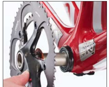
Figure 27. Sliding the axle through the bearings
