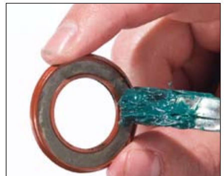
Figure 24. Greasing the bearing covers
