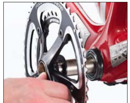
Figure 51. Sliding the axle through the bearings
