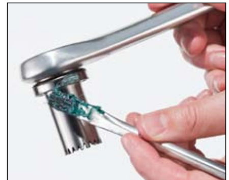
Figure 42. Greasing the bearings
