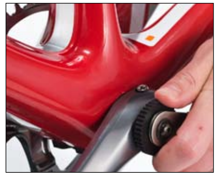
Figure 37. Pressing the crank arm onto the axle
