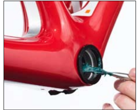
Figure 43. Greasing the bearing cups
