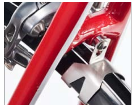
Figure 15. Fender bridge clip held by interior screw
