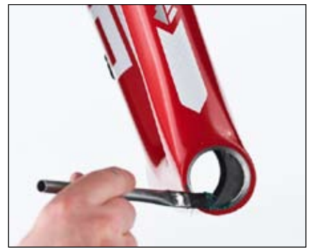
Figure 7. Greasing upper bearing saddle
