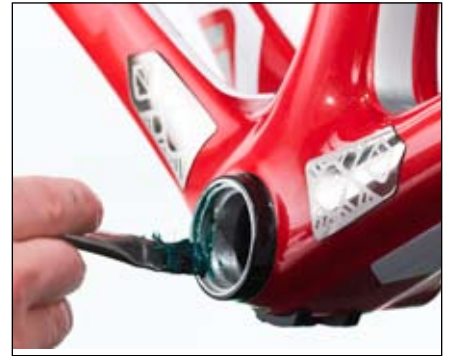
Figure 48. Greasing the bearing and the frame saddle
