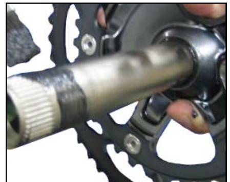
Figure 50. Greasing the axle
