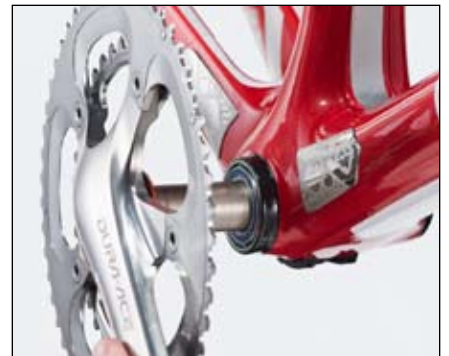
Figure 35. Sliding the axle through the bearings
