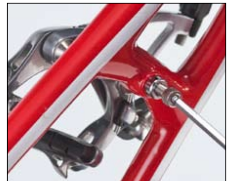
Figure 14. Removing interior screw from brake nut
