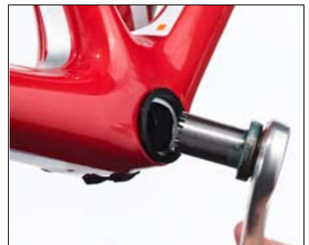
Figure 45. Inserting the non-drive side axle
