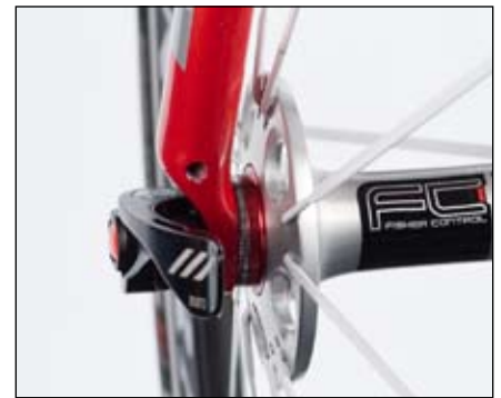
Figure 19. Large diameter hub end faces mate to oversized fork tips
