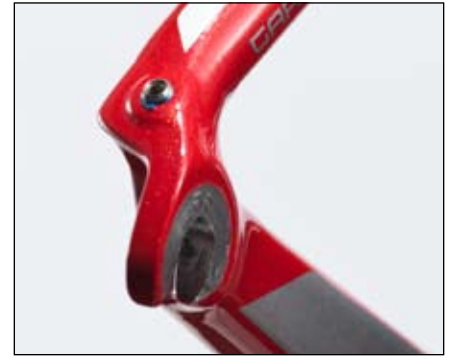
Figure 12. Threaded hole in left rear dropout
