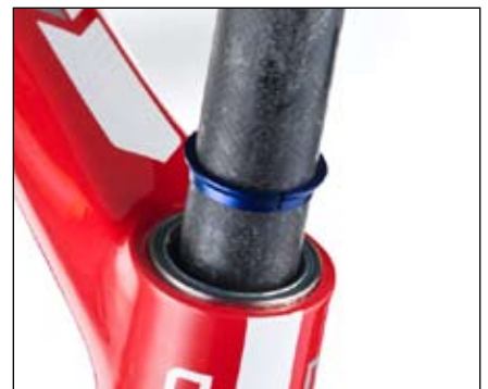
Figure 9. Slide the centering washer onto the steerer
