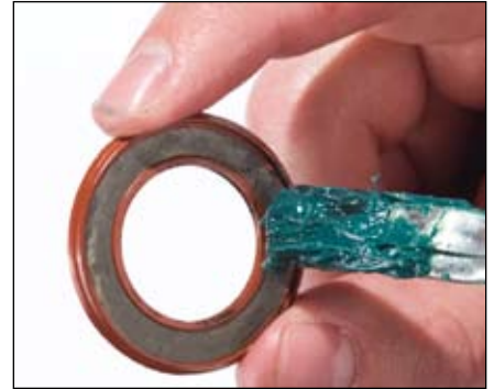
Figure 32. Greasing the bearing covers
