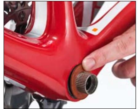
Figure 36. Pressing in the second bearing cover
