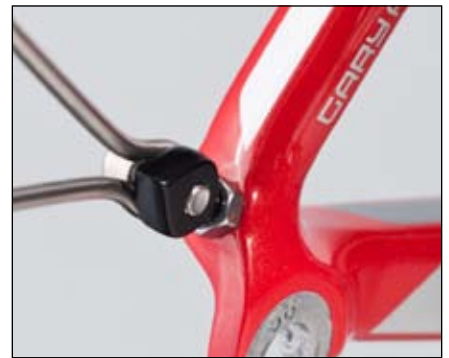
Figure 17. Fender strut attached to eyelet
