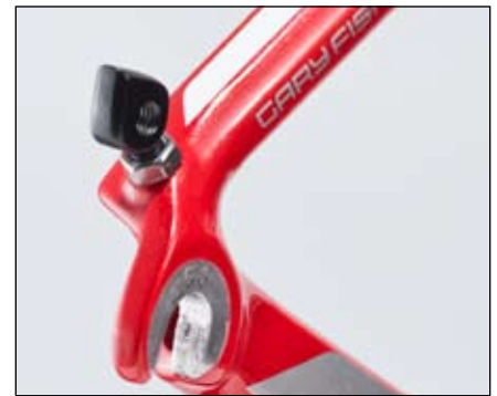
Figure 13. Eyelet with locknut installed in dropout
