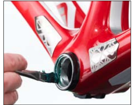
Figure 30. Greasing the bearing and the frame seat
