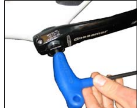
Figure 52. Pressing the crank arm onto the axle
