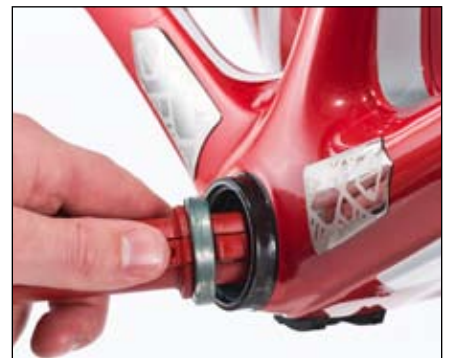
Figure 23. Pressing the bearing into the frame
