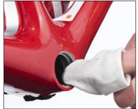
Figure 39. Cleaning bonding surfaces with an alcohol wipe
