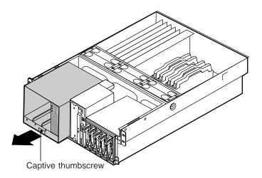
**8** Tilt the power supply forward and lift it up and back to clear the tab on the bottom of the chassis.
