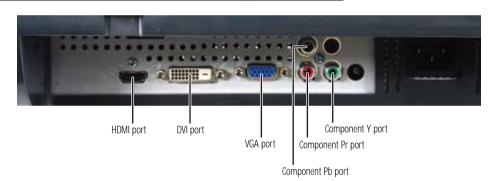
3 Make sure that your computer is turned off, then connect the other end of the video cable to the matching video port on the back of your computer.
