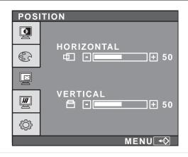
**HORIZONTAL.** Moves the display image left and right. **VERTICAL.** Moves the display image up and down.
