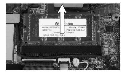
**3** Hold the replacement module at a 30-degree angle and press it into the empty memory slot. This module is keyed so it can only be inserted in one direction. If the module does not fit, make sure that the notch in the module lines up with the tab in the memory bay.
