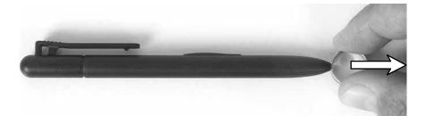
**2** Insert a new point and apply slight pressure to set it in place.
