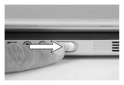
The power switch is preset to On/Off mode. However, you can also set it to function in Standby/Resume mode.
