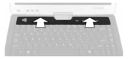
**6** Press down on the bezel in several places to make sure it is correctly mounted. The bezel is correctly mounted when you can run your finger along the bezel and find no loose spots. The bezel should be flat all the way across.
