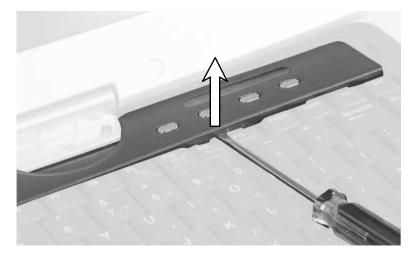
**12** Remove the bezel from your convertible tablet PC by pulling the bezel toward you and at the same time lifting its front to clear the keyboard. You will hear small snapping sounds as the bezel comes away from your convertible tablet PC. Be careful not to break off the tabs found on the bottom of the bezel.
