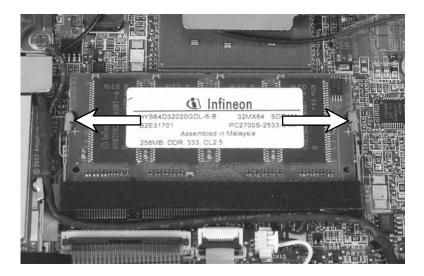
**2** Pull the memory module out of the slot.
