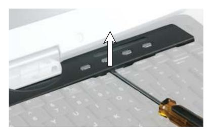
**9** Remove the bezel from your convertible tablet PC by pulling the bezel toward you and at the same time lifting its front to clear the keyboard. You will hear small snapping sounds as the bezel comes away from your convertible tablet PC. Be careful not to break off the tabs found on the bottom of the bezel.
