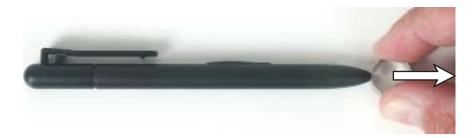
2 Insert a new point and apply slight pressure to set it in place.
