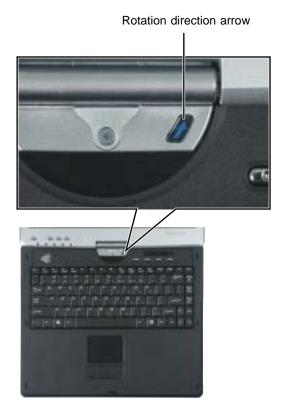
**3** Rotate the LCD panel in the direction of the rotation direction arrow until the panel is backwards. The panel *soft-locks* into the final position.
