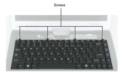
11 Lift the back edge of the keyboard, then slowly rotate it toward you so it lies **keys-down** on top of your convertible tablet PC. Be careful not to damage the LCD panel, or unplug the keyboard ribbon cable.
