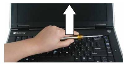
12 Pull the cover off the notebook. Be careful to not damage the LCD panel.
