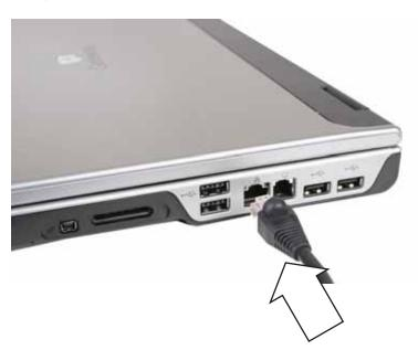
2 Insert the other end of the network cable into a cable modem, DSL modem, or Ethernet network jack.
