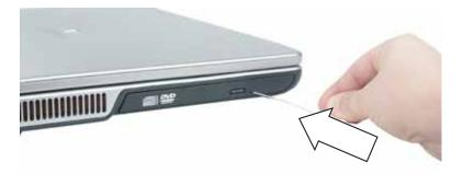
10 Carefully slide the drive out of the drive bay.
