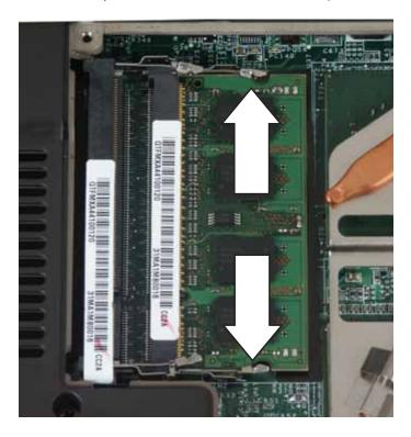
8 Pull the memory module out of the slot.
