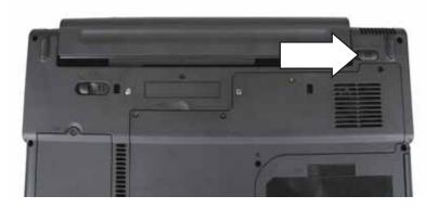
5 Slide the battery release latch, then slide the battery out of the notebook.
