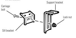
**B** Open the window and mark the centerline of the window stool. Measure and mark 11" to the left and right of the centerline.
