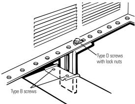
**D** Adjust the carriage bolts and the lock nuts in each support so that the case is installed with a slight downward tilt (about 1/4") toward the outside. Tighten the bolts.
