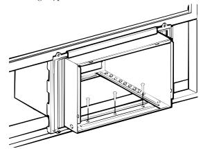
**F** Pull the accordion panels to each window sash track. Attach them on each side to the window sash and the window stool using 4 type C screws.
