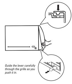
**D** Lift the inlet grille and secure the front frame with a type A screw. Lower the inlet grille into place.
