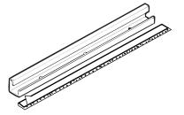
D Install the top mounting rail with 3 type A screws on the inside of the case. Insert the frames for the accordion panels into the top mounting rail and the frame guides. Attach the accordion panels to the side of the case using 5 type A screws.
