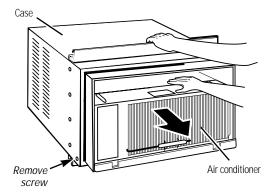
**D** Slide the air conditioner out of the case by grasping the rear of the evaporator cover and pulling forward while bracing the case.
