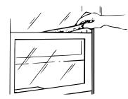
Slide the air conditioner into the case and Β replace the front grille. Install the two ground/anti-theft screws removed at the beginning of the installation.
