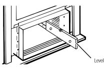
**NOTE:** When finished, use a level to make sure the case tilts to the outside 1/4" minimum. This prevents water from entering the room.
