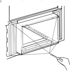
Attach the window locking bracket with a С 5/8" screw.
