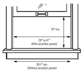
Window opening dimensions are for a standard double-hung
