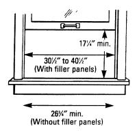
Window opening dimensions are for a standard double-hung window.
