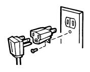
This is a temporary method. UL-listed adapters are available at most hardware stores. Because most 2-prong outlets are not grounded, we strongly advise against using an adapter plug. However, a temporary connection may be made where local codes permit and if the 2-prong wall outlet is properly grounded.
