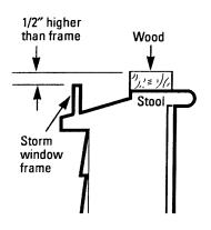
A storm window frame will not allow the air conditioner to tilt towards the outside and will keep it from draining properly. To adjust for this, attach a piece of wood to the stool.
