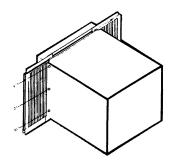
**3** Peel the backing off the bottom window gasket and place onto the backside of the window stool.
