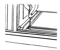
**3** Assemble the 2 leveling bolts and nuts to the support brackets.
