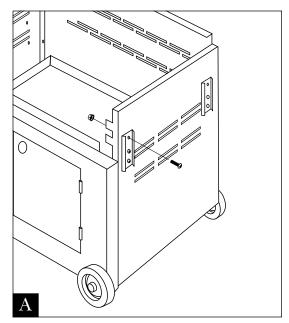
• Remove the top screw in the front shelf slide on the left and right sides. Retain screws. NOTE: One shelf is marked "R/H Shelf". Be sure to use that shelf on the right side of the cart.
