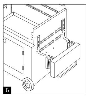
• Slide shelf supports up and into the channels on the sides of the cart.
