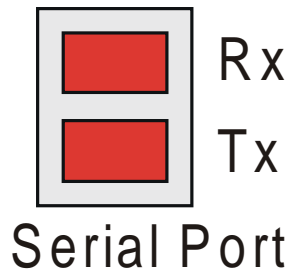
Figure 5.4 – Automation Equipment Port Receive & Transmit LEDs The LED's flash when the TIU20X is communicating with the AE.
