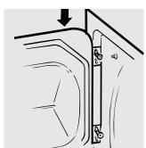
Rotate the door 180°. Insert it on the opposite side of the opening by moving the door *IN* and *DOWN* until the top hinge and the bottom hinge are resting on the top screws inserted in step 1.
