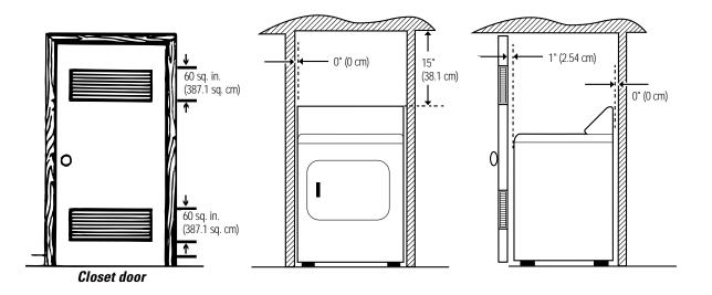
Dryer **MUST** be exhausted outside (outdoors, not beneath the mobile home) using metal ducting that will not support combustion. Metal ducting must be 4'' (10.16 cm) in diameter with no obstructions. Rigid metal duct is preferred.
