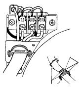
**WARNING:** Do not make a sharp bend or crimp wiring/conductor at the connections.
