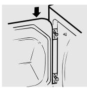
7 Remove the remaining screws from the side of the opening from which the door was removed. With these screws secure each hinge at the bottom.
