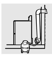
Inspect and clean the dryer exhaust ducting at least once a year to prevent clogging. A partially clogged exhaust can lengthen the drying time. To clean the exhaust duct follow these steps:
