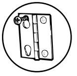
Z Loosen top screw from each hinge on the dryer face halfway. With one hand holding the top of the door and the other hand holding the bottom, remove the door from the dryer by lifting it **UP** and **OUT**.
