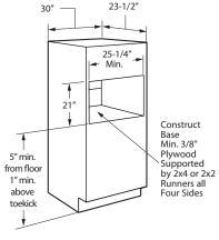
• Oven overlaps will conceal cut edges on all sides of the opening. **Note:** PSB1200/1 series Advantium can be installed below GE/GE Profile non-downdraft gas and electric cooktops. It CANNOT be installed below induction or Monogram (2GU3841385) gas cooktops.
