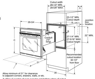
A=Allow 1" overlap of oven over top and bottom edges of cutout. B=Allow 11/16"-3/4" for overlap of oven over side edges of cutout. C=28-1/4" without trim and 28-3/4" with trim.
