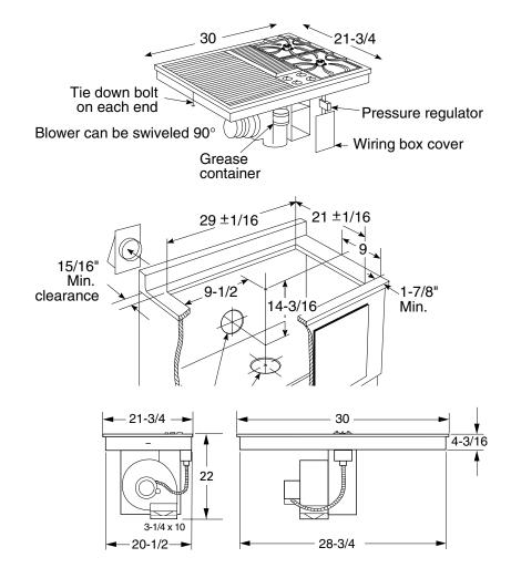
\*Note: A 8" minimum spacing to adjacent side wall is required
