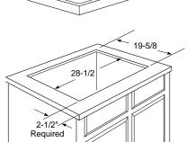
\*Depth of unit at conduit location (rear) is 4-5/8"
