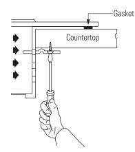
**Note:** If the cooktop is installed in a 36" base cabinet, the mounting brackets cannot be used because of interference with the cabinet sides. In this case, the cooktop can be secured to the cabinet with angle brackets (not supplied).
