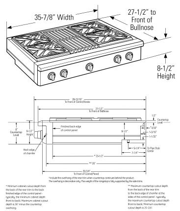
Allow 8" free space below the top surface of countertop. Allow additional clearances below the burner box to install the regulator and make house gas supply connections. Use a 90° elbow to route the gas connections and limit interference with drawers or other cabinetry.
