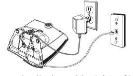
Plug the power supply cord into the power jack on the bottom of the base and the other end into an electrical outlet. The in use/charge indicator (on the base) turns on to indicate the battery is charging when the handset is on the cradle. Allow the phone to charge for 16 hours prior to first use. If you don't properly
