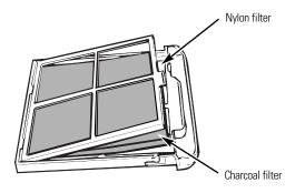
Vacuum the nylon filter or wash with water. Make sure it is dry before replacing it.
