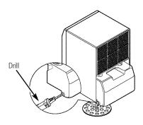
**NOTE:** The nozzle cannot be fixed after puncture. Use an ordinary garden hose cap (not included) to reclose if necessary.
