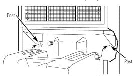
Make sure the bucket is locked securely in place by pressing down on the upper back edge of the bucket. It will be firmly seated when properly installed.
