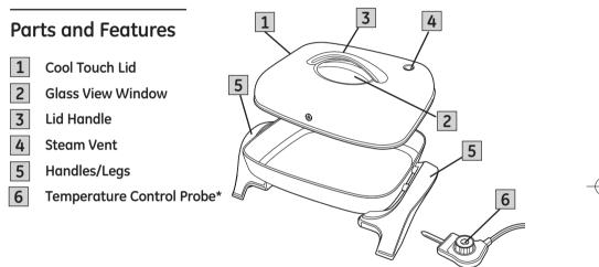
\*NOTE: Only use with the Temperature Control Probe model that is marked on the bottom of the temperature control probe guard.
