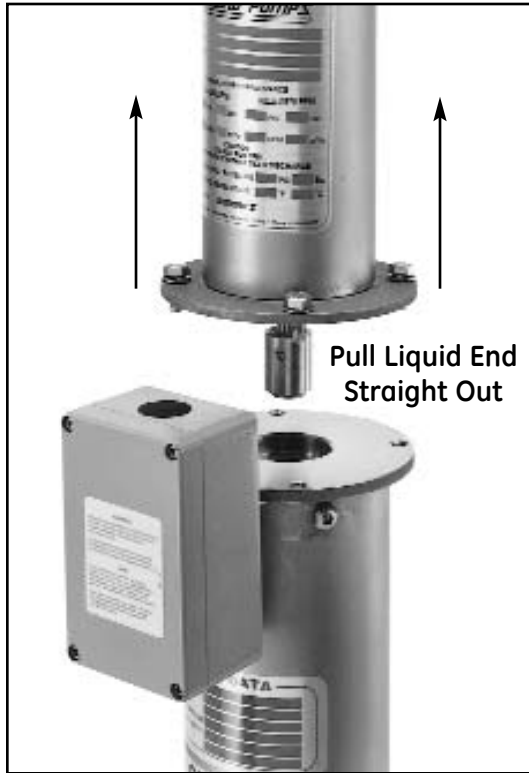
Figure 6.9 Removing Liquid End (QS2825V Shown)
