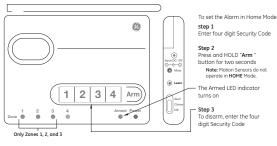
**Step 1 -** Enter your four digit Security Code. **Step 2 -** Press/hold the Arm button for two seconds. The red Arm LED indicator will turn on. The system is now Armed.
