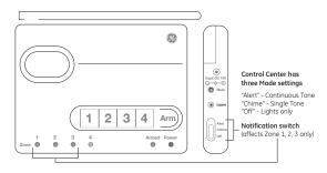
**Zone 4** is designated for detected Alerts only. Use Zone 4 for areas you wish to continuously monitor, but don't want to trigger the alarm (e.g. notification of water leaks, garage door is up, back gate left
