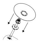
**3.** Firmly push the cover ring onto the securing collar snap clips until each clip snaps into place.
