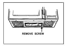
To replace cooktop light in hood, first disconnect power at main fuse or circuit breaker panel or pull plug. Remove screw on right side of light compartment cover and lower cover until it stops.
