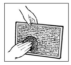
To clean grease filter, soak, then agitate filter in hot detergent solution. Don't use ammonia or other alkali because it will darken metal. Light brushing can be used to remove embedded dirt. Rinse, shake and remove moisture before replacing. Filters should be cleaned at least once a month. Never operate your hood without the filter in place. In situations where flaming might occur on surfaces below hood, filter will retard entry of flames into the unit.
