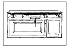
Next, remove the single screw located above door near center of oven that secures light housing. Remove bulb and replace with a 30-watt GE bulb (Part No. WB2X4235) available from your GE supplier. Secure light housing with screw.
