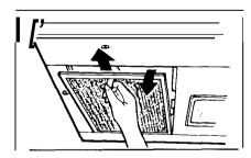
Then pull filter downward and to the front. The filter will drop out.
