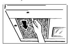
To remove grease filter, grasp the "finger hold" on the filter and slide to the rear.
