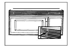
To replace your oven light, first disconnect power at main fuse or circuit breaker or pull plug. Remove the top grill by taking off 3 screws which hold it in place.
