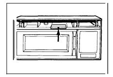
Next, remove the single screw located above door near center of oven that secures light housing. Remove bulb and replace with 30-watt incandescent bulb (Part No. WB02X4235) available from your GE supplier. Secure light housing with screw.
