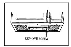
To replace cooktop light, first disconnect power at main fuse or circuit breaker panel or pull plug. Remove screw on right side of light compartment cover and lower cover until it stops.
