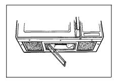
Be sure bulbs to be replaced are cool before removing. Break the adhesive seal by gently unscrewing the bulbs. Replace with 40-watt incandescent bulbs (Part No. WB02X4253) available from your GE supplier. High intensity 40-watt bulbs (40S11N/1) which are available in supermarkets and hardware stores may also be used for replacements. Raise light compartment cover and replace screw. Connect electrical power to microwave oven.
