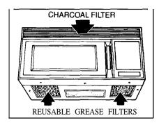
Your microwave oven has two reusable metal filters to help remove grease from the air and a disposable charcoal filter to help remove smoke and odors caused by cooking with your range. When the fan is operated, air is drawn up through the filters and then recirculated.
