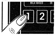
Step 2: Touch 1, 5, 0 and 0 for defrosting time. 15:00 appears on readout display. (Defrosting is automatically set on Power Level 3 but can be changed by touching POWER LEVEL pad and the new Power Level.)
