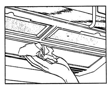
Clean off the grease and dust on hood surfaces often. Use a warm detergent solution. About 1 tablespoon of ammonia may be added to the water. Take care not to touch the filters and enameled surfaces with this. Ammonia will tend to darken metal.
