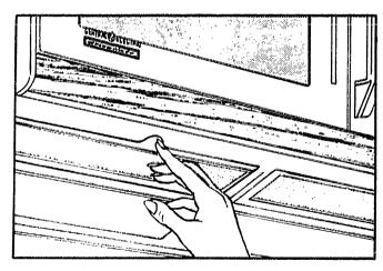
To remove grease filter, grasp the "finger hold" on the filter and push to the rear. The filter will drop out.
