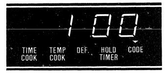
2. Light over Code shows on display. Readout displays internal food temperature.
