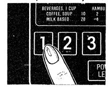
STEP 2: Enter the proper code into Cook Code control. For example, a recipe calling for 12 minutes cooking time at Power Level 10 would be 120. 120 appears on the display panel.
