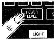
Step 4: Touch POWER LEVEL pad. Touch 5 for MEDIUM power. P-5 shows on display and then display reverts back to set finished temperature.
