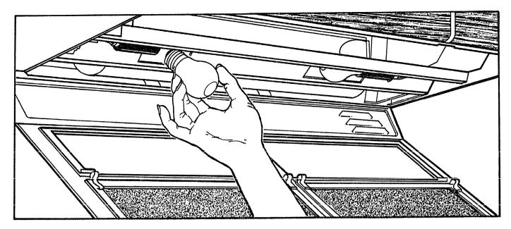
To replace hood lamp, first disconnect power at main fuse or circuit breaker panel or pull plug. Remove 2 screws from each side of lower panel and 3 screws from front edge. Lower panel until it rests on range below. Be sure bulb to be replaced is cool
