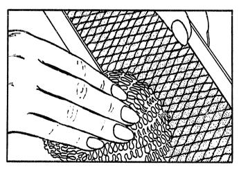
Soak, then agitate filter in hot detergent solution. Don't use ammonia or other alkali because it will darken metal. Light brushing can be used to remove embedded dirt. Rinse, shake and remove moisture before replacing. Filters should be cleaned at least once a month. Never operate your hood without the filter in place. In situations where flaming might occur on surfaces below hood, filter will retard entry of flames into the unit.
