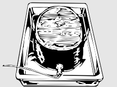
The temperature probe has a skewer-like probe at one end and a plug at the other end that goes into the outlet in the oven.
