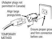
Ensure proper ground and firm connection
