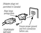
at most local hardware stores. The larger slot in the adapter must be aligned with the larger slot in the wall receptacle to provide proper polarity in the connection of
