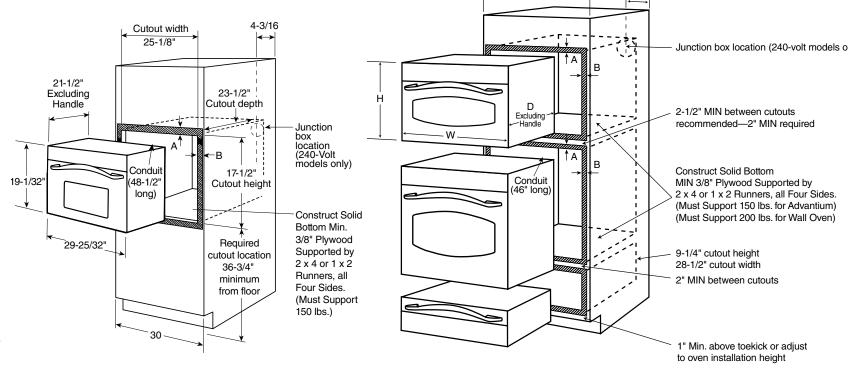
A=Allow 1" overlap of oven over top and bottom edges of cutout. B=Allow 11/16"-3/4" for overlap ov oven over side edges of cutout.
