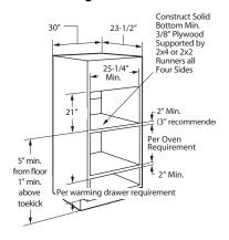
\* For existing cutouts, a maximum width of 28-1/2" is acceptable. If the opening is slightly wider, secure a furring strip on each side of the cutout for securing the oven.
