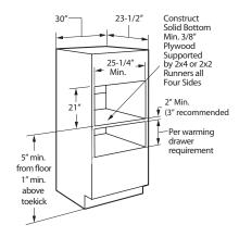
\* For existing cutouts, a maximum width of 28-1/2" is acceptable. If the opening is slightly wider, secure a furring strip on each side of the cutout for securing the oven.
