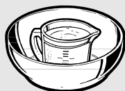
How to test for a microwave-safe dish.
