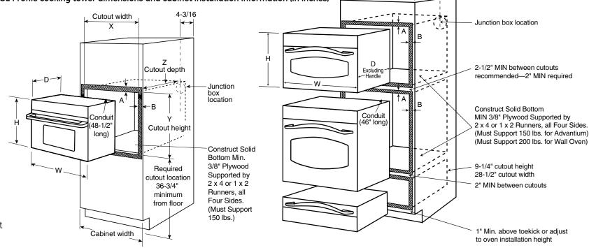
A=Allow 1" overlap of oven over top and bottom edges of cutout. B=Allow 11/16"-3/4" for overlap of oven over side edges of cutout.
