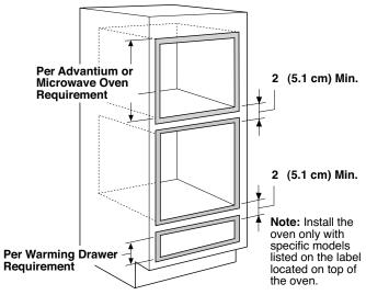
The solid bottom or runners must be level with the bottom of the cutout, or the bottom trim may not install correctly and could interfere with the door opening. If the cabinet does not have a solid bottom, two braces or runners must be installed level with the bottom of the cutout to support the weight of the oven. The runners and braces must support 200 lbs. (90 kg).
