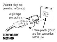
**ACAUTION:** Attaching the adapter ground terminal to the wall receptacle cover screw does not ground the appliance unless the cover screw is metal, and not insulated, and the wall receptacle is grounded through the house wiring.
