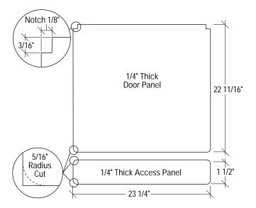
Cut 1/4" thick door panel: 23-1/4" wide, 22-11/16" high. Cut 1/4" thick access panel: 23-1/4" wide 1-1/2" high. Cut edges of the panels will be concealed by the trim.
