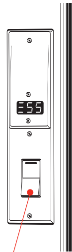
On/Off switch for interior ceiling lighting
