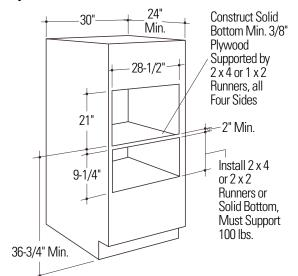
Note: Additional clearance between the cutouts may be required. Check to be sure the oven supports above the warming drawer location do not obstruct the required interior 23-1/2" depth and 9-1/4" height. See installation instructions for details.
