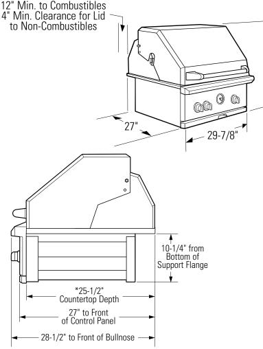
\*The weight of the grill is fully supported by the side trims. The back of the grill overlaps the back edge of the cutout.
