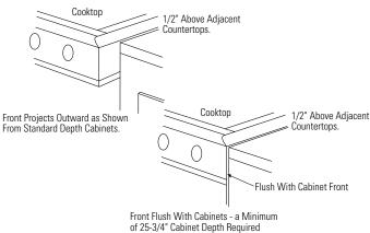
NOTE: These cooktops require 8" free space below the countertop to house the cooktop burner box. Allow additional clearances below the burner box to install the regulator and make house gas supply connections. Use a  $90^{\circ}$  elbow to route the gas connections and limit interference with drawers or other cabinetry features.
