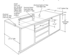
**Note:** When installing warming drawer with a cooktop, allow a 2" minimum from cooktop burner box bottom to top of cut-out.
