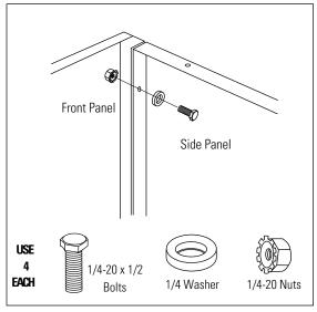
• Stand the assembly up and bolt the front panel to the side panels with bolts, washers and nuts as shown. (2 on each side).
