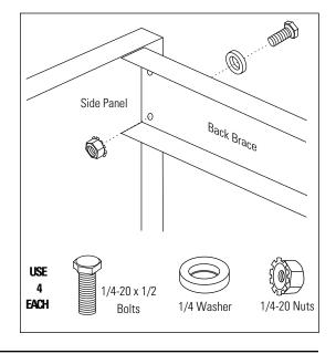
Step 6 Check Panel Alignment, Tighten Assembly
