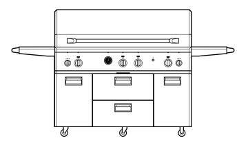
Monogram grills are factory-set for Natural or LP gas operation. Be sure to order the correct model for the installation situation.
